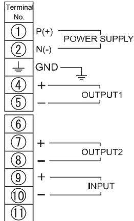
With 3-wire sensor power supply:
