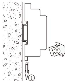
Push the slide clamp downward with a flat-head screwdriver bit or the like (①), and pull the lower part of the socket toward you (②).
