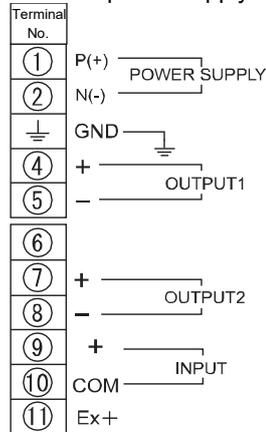
With 2-wire sensor power supply:
