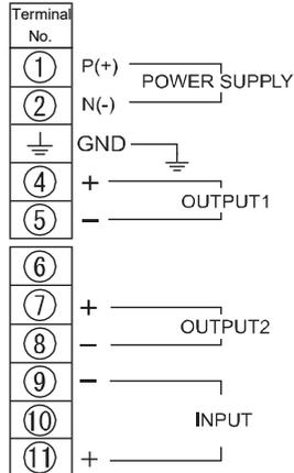
For models with 2-wire sensor power supply, the connections may vary depending on the type of the sensor used.
